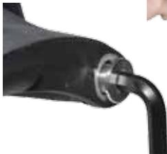
2. Loosen main screw minimum 1/4" (6mm).
